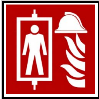
Figur 5.12.1 Piktogram for brandmandselevator.
