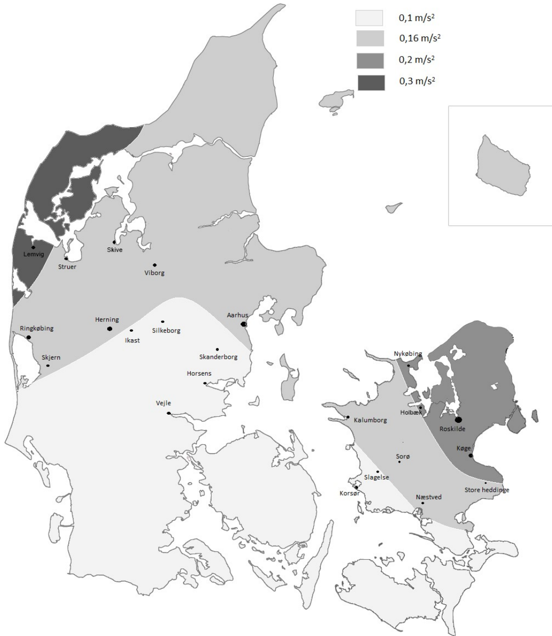
Figure D.2 DK NA: Values of design ground acceleration, a_g The values are given in m/s^2 .
